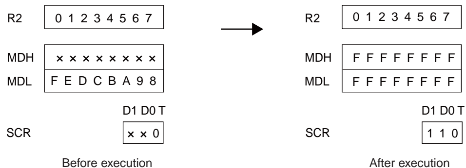
Figure 6.6-1 Example of execution of signed division
